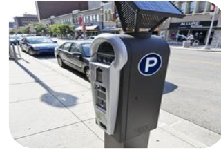
PV Parking Meters
